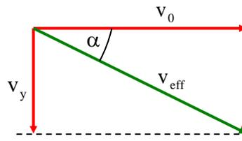
$$v_{\text{eff}} = \sqrt{v_0^2 + v_y^2} = \sqrt{v_0^2 + 2gh_0}$$
